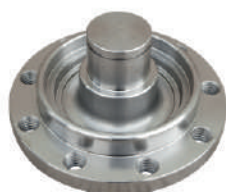
Stub Axle (9 Hole) Part No. NR 3078
